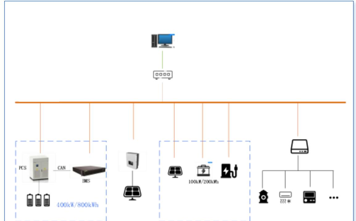
The communication topology of the energy management system (EMS) is divided into two levels: the upper level is the overall centralised video monitoring system, and the lower level is the equipment: a 500 kW storage inverter, battery management system (BMS), environmental monitoring equipment, fire protection system, air conditioning or access control system, etc., all connected to a video monitoring system.
